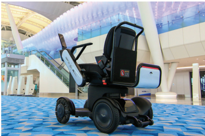
Figure 27. Autonomous wheelchair that operates in the departure security area of each terminal at Tokyo Haneda Airport [27]
